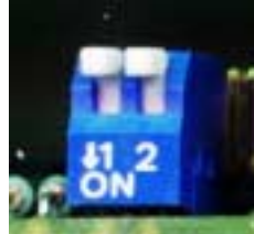
Adapter MD33D DIP-switch S1
